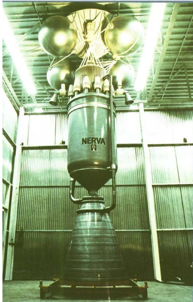
A small nuclear reactor powered this NERVA rocket. NERVA used liquid hydrogen propellant.
